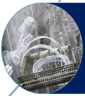
For isolator, all parts/components are to be sterilized in autoclave / other suitable means and to be transferred inside the isolator. It can be semi assembled and without removal of bacterial barrier paper/Tyvek wrapper from critical contact parts.
