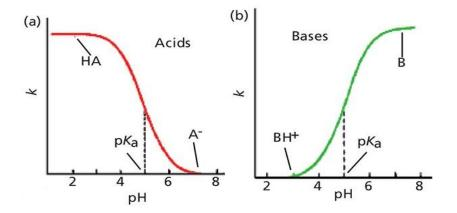
Figure 1: Retention behavior/factor (k) versus pH; (a): Acidic compounds (b): Basic compounds
