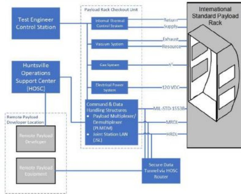
Extensive testing is performed for qualification and acceptance testing prior to on-orbit operations by providing access to resources in an ISS-analogous environment
