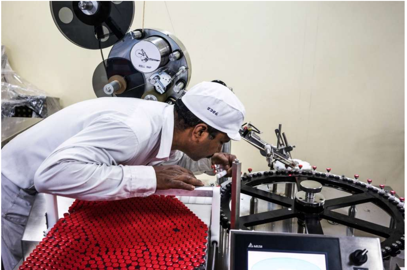
An employee checks a vaccine vial labeling machine at a Serum Institute of India pharmaceutical plant in Pune, India in 2015. The Institute working with AstraZeneca to produce a COVID-19 vaccine developed by Oxford.
